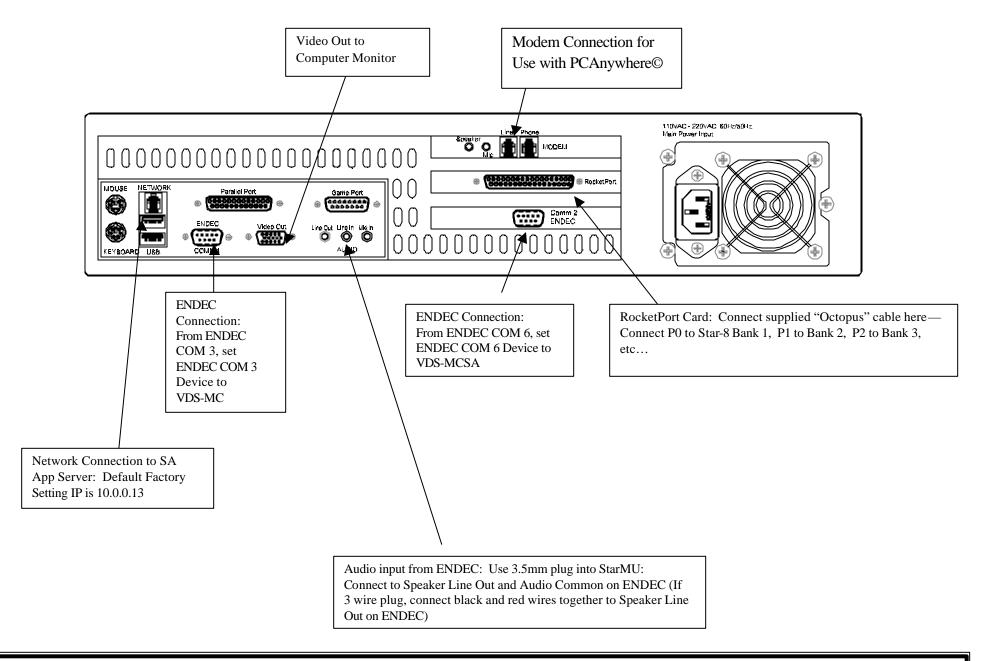
Note that the ENDEC connects to the StarMU with a supplied Null Modem Cable only. Other cables will not make proper link. ENDEC can connect to either Comm 1 and/or Comm 2. The default factory setting is Comm 1 to connect to ENDEC COM 3 (Analog for Star-8 Channels), and Comm 2 to connect to ENDEC COM 6 (Digital for Scientific Atlanta<sup>TM</sup> App Server System)
