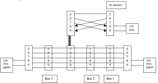
Above diagrams show connection of 4 STAR-8 boxes for a total of 32 channels.
