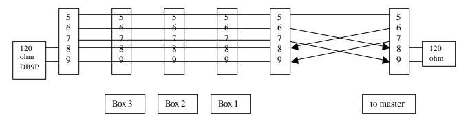
If you must connect the master unit somewhere in the middle of the chain, then you should use the null modem type cable described above between the cable position designated for the master and the master unit. Note that when you provide the master at a mid point connection then you should provide two terminating DB9P connectors, one at each end of the ribbon cable, each one with a 240 ohm termination resistor across pins 8 and 9.
