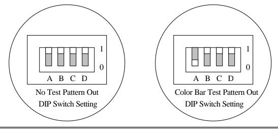
The 100% color bar test pattern generation may be selected on or off by the user. Place "A" switch to the "0" position to generate the test pattern. The test pattern will output in the standard and format selected by the remaining switches
