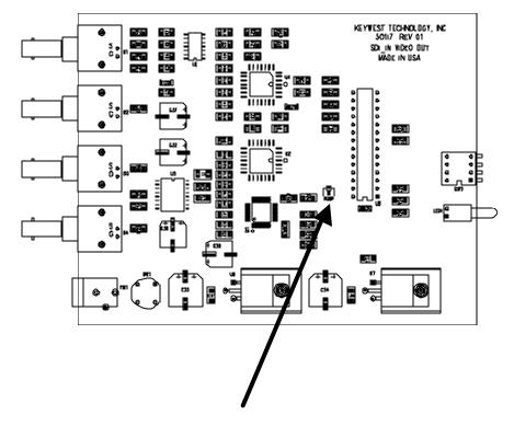
Adjust R29 (shown above) for overall composite video output level
