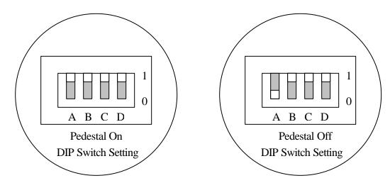
The 7.5 IRE pedestal may be selected on or off by the user (if requested at time of order). This feature is a special request item. Software can be changed for either mode, but requires a special request to Keywest Technology for replacement processor.
