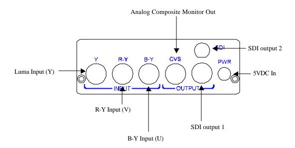
All video connections to be made with industry standard BNC connectors
